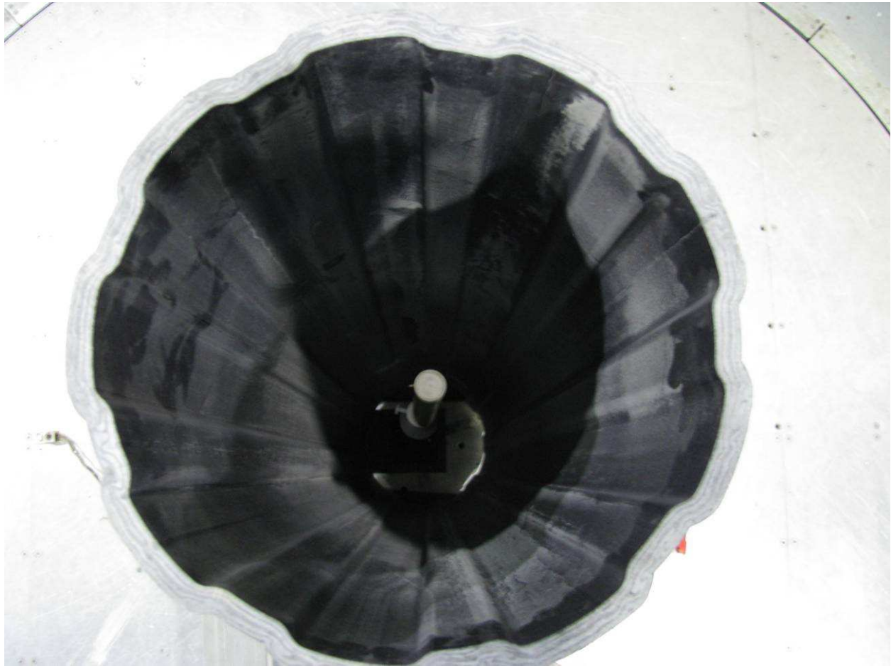
Photograph Showing the Transmitting Antenna Centered Within the Test Sample (Taken From Above)
